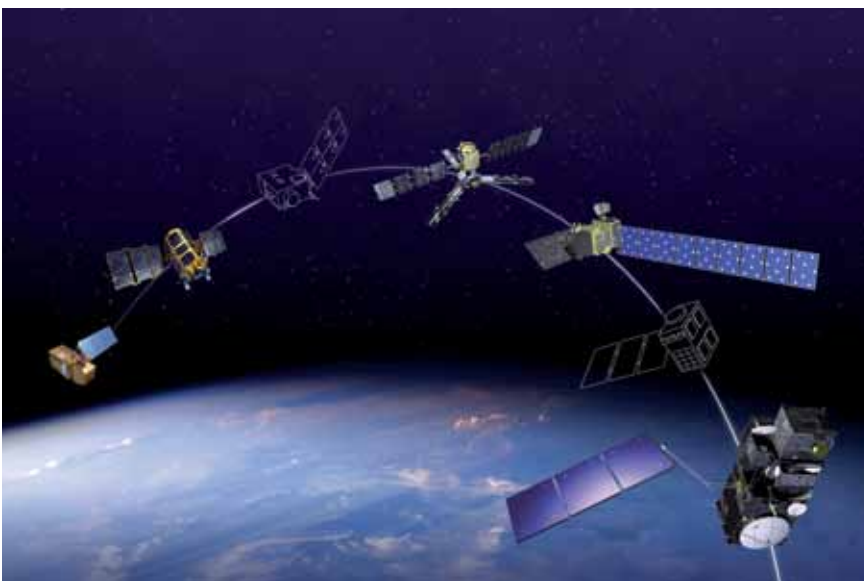
Figure 4.3. The construction of a virtual constellation of satellites from different space agencies. International collaboration is needed for the cost-effective and optimal design of a global integrated observing system. Such a system could involve virtual constellations, as illustrated here, or formation flying and convoys. International collaboration should extend to open access to data (from publicly funded satellite missions and projects at least), data sharing, data quality assessment and interoperable data processing systems.
